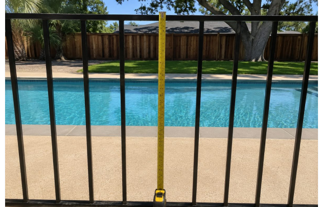
Fence measured at 60 in., vertical bars under 4 in. apart, no footholds on the outside.
